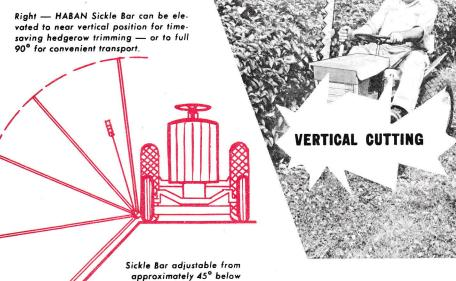
horizontal to near vertical position for multi-angle mowing.
